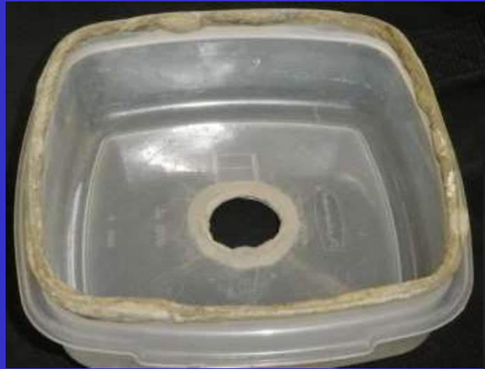
Sample-box adaptor with rope caulk at perimeter openings
